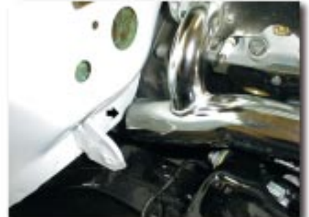
717052 Passenger Side header. Firewall-to-floorboard seam must be bent over for exhaust clearance.
