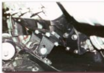
713111 motor mounts installed using the stock V6 rubber mounts.
