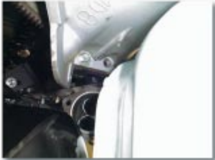
Transmission ear should be removed to aid in exhaust clearance. (This transmission has not be modified).
