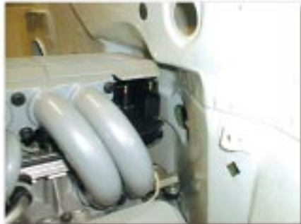
Distributor clearance off the firewall using 713111 mounts.
